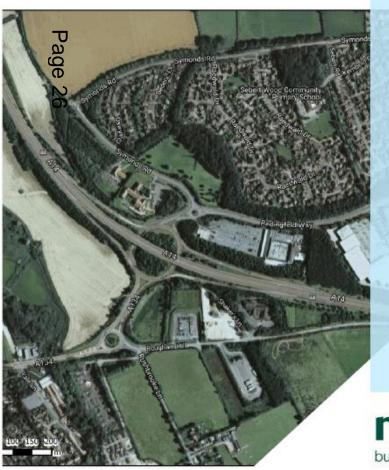
→ Poor layout, short slip roads and lack of capacity leads to significant congestion and queueing, which extends back onto the A14 main carriageway.
